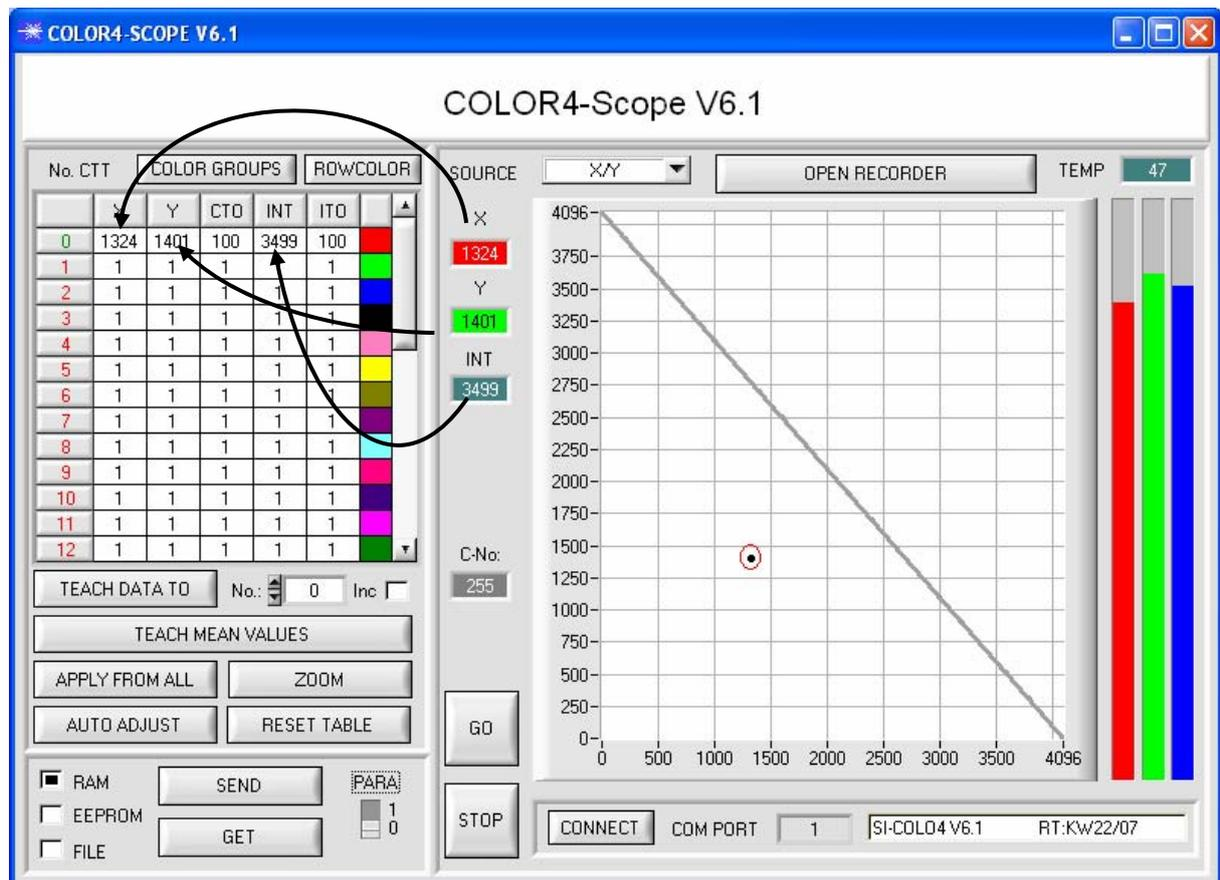
Now press the SEND button again to inform the sensor about the taught color. Then activate the GO mode again. When the sensor recognizes a line vector (color), the responding line number is visualized in C-No.: at the software user interface. The value 255 means that none of the taught colors has been recognized.
